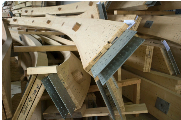
Figure 3. 11 miles of compound curved glulam pieces each digitally fabricated from a unique glulam blank.
